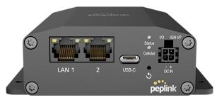
Max Adapter V2 has both a USB-C port (ostensibly for power and/or network data) and two Ethernet ports for data. It also comes with an external AC power adapter. The simplest way to use the MAX Adapter with ACCESS is to power the Peplink device from its external power supply and attach an Ethernet cable between the Max Adapter's "LAN1" port and the codec's Ethernet port. You won't get any status feedback on the UI of the ACCESS, as it will appear just like a normal Ethernet LAN.
