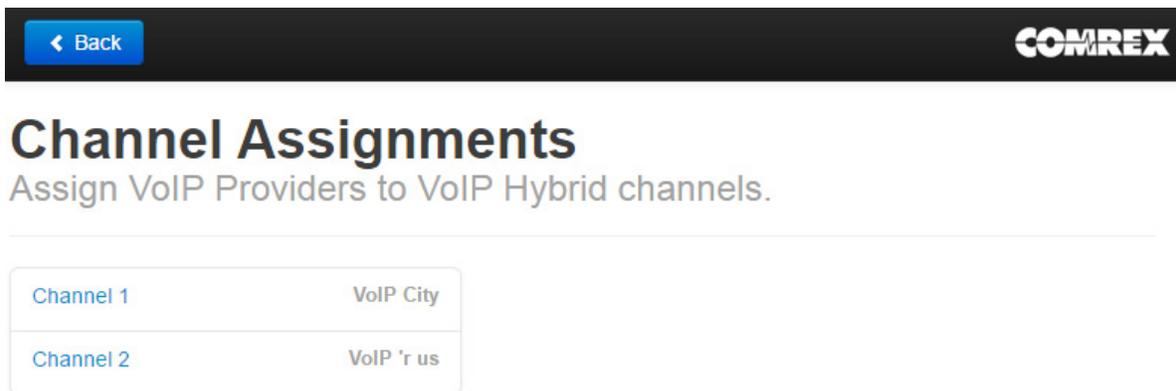
The figure shows each channel assigned to a different provider. Each channel could also be assigned to the same provider, and the usual behavior is for calls to "hunt" between the channels (first call on channel 1, second on 2).
