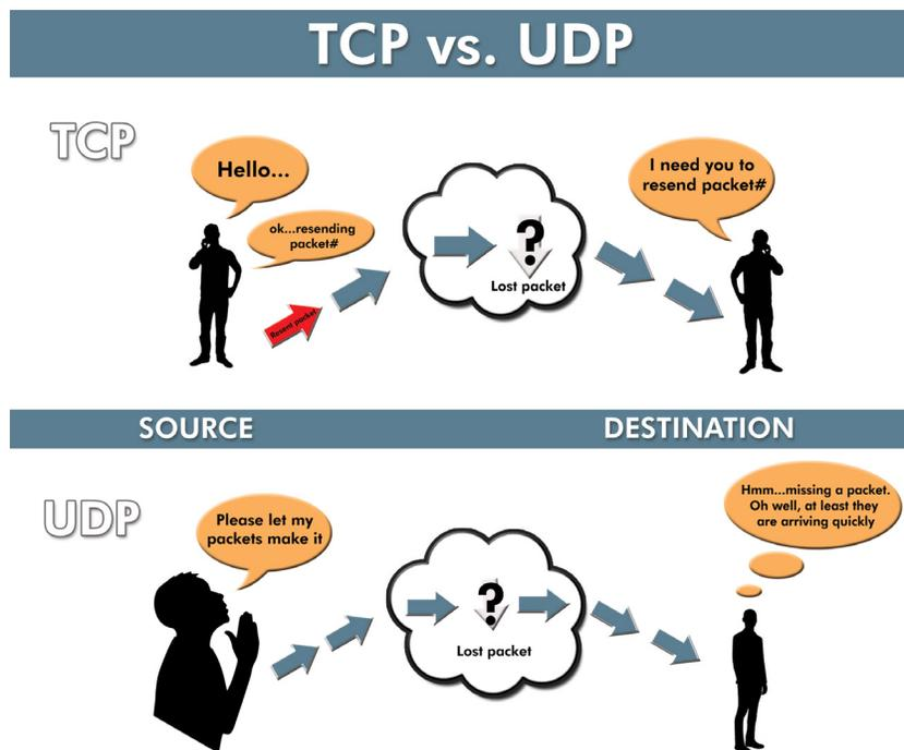
Packets sent on IP networks will include a destination IP address/port combination, and a source IP address/port combination. These act like the destination and return address on an envelope, and allow the packets to be responded to over the network.
