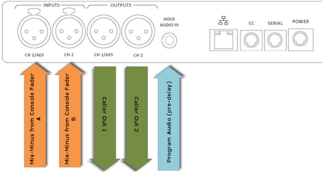
Finally, VH2 is capable of behaving like two, completely independent products for use in two, unrelated studios. This is shown below.
