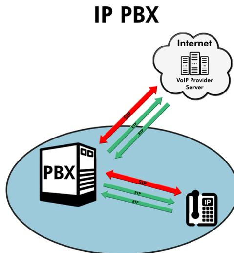
It's important to understand that the SIP protocol does not carry any actual voice between devices-- it simply instructs devices to create separate RTP sessions in each direction. RTP streams are created and destroyed based on commands contained in SIP messages when calls are made or received.
